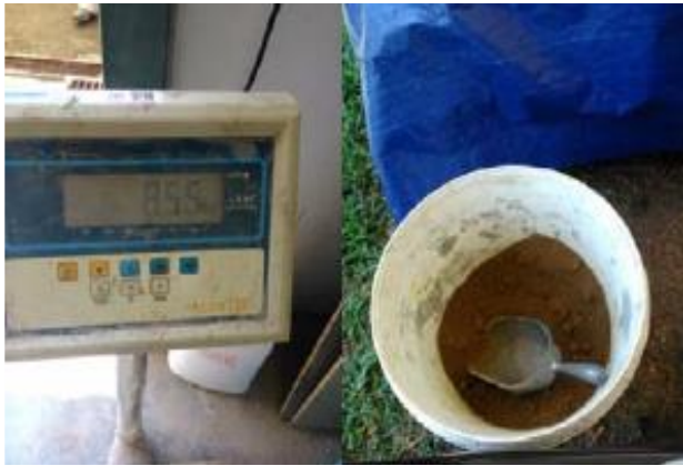
Figure 1 The example of mixing process during the preparation of 5% cement content in 9 kg soil-cement mixture
