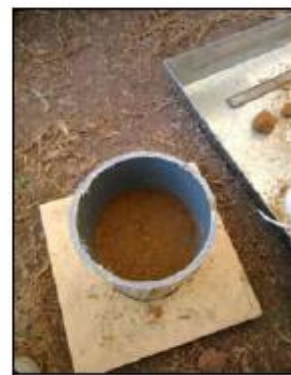
Figure 2 Throughout the process of compacting soil-cement mixture in the PVC cylinder
