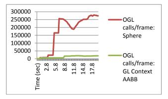
Figure 9Comparison of OpenGL function cal per frame for bounding sphere hierarchy and AABB hierarchy
