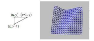
Figure 1 Particles arrangement for cloth structure
