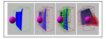
Figure 6 The Axis Aligned Bounding Box (AABB)
