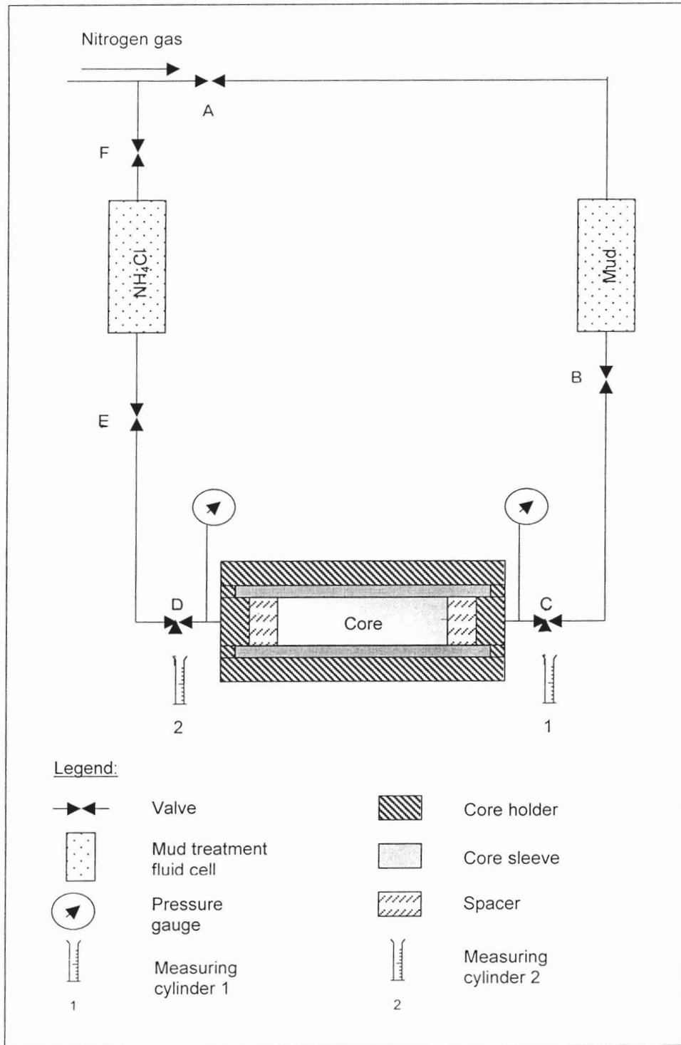
**Figure 1** Schematic diagram of the formation damage system
