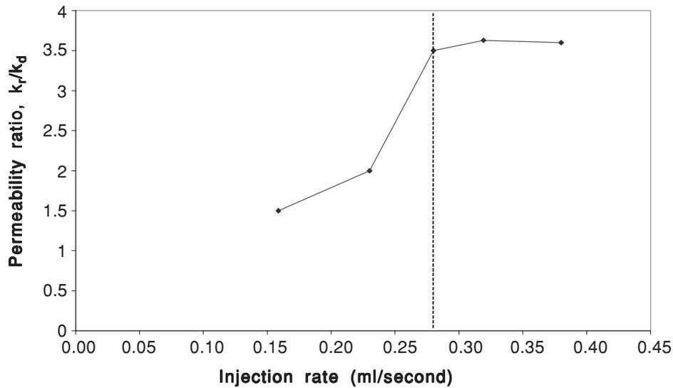
**Figure 5** Effect of injection rate on the permeability ratio
