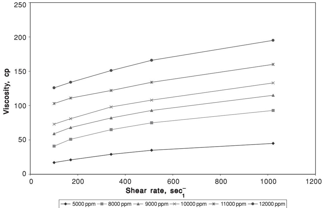
Figure 3 The effect of xanthan gum concentration on gel viscosity at various shear rates
