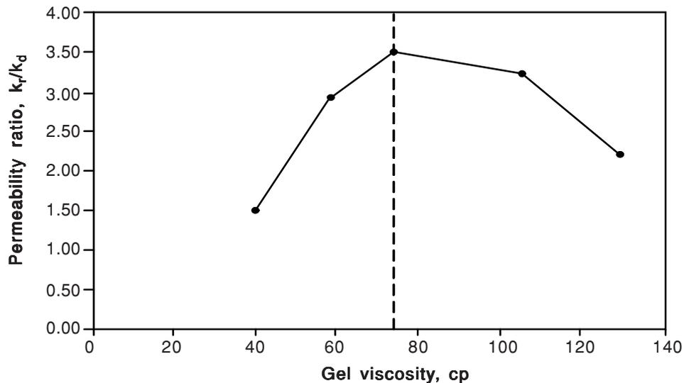
**Figure 6** Effect of gel viscosity on the permeability ratio
