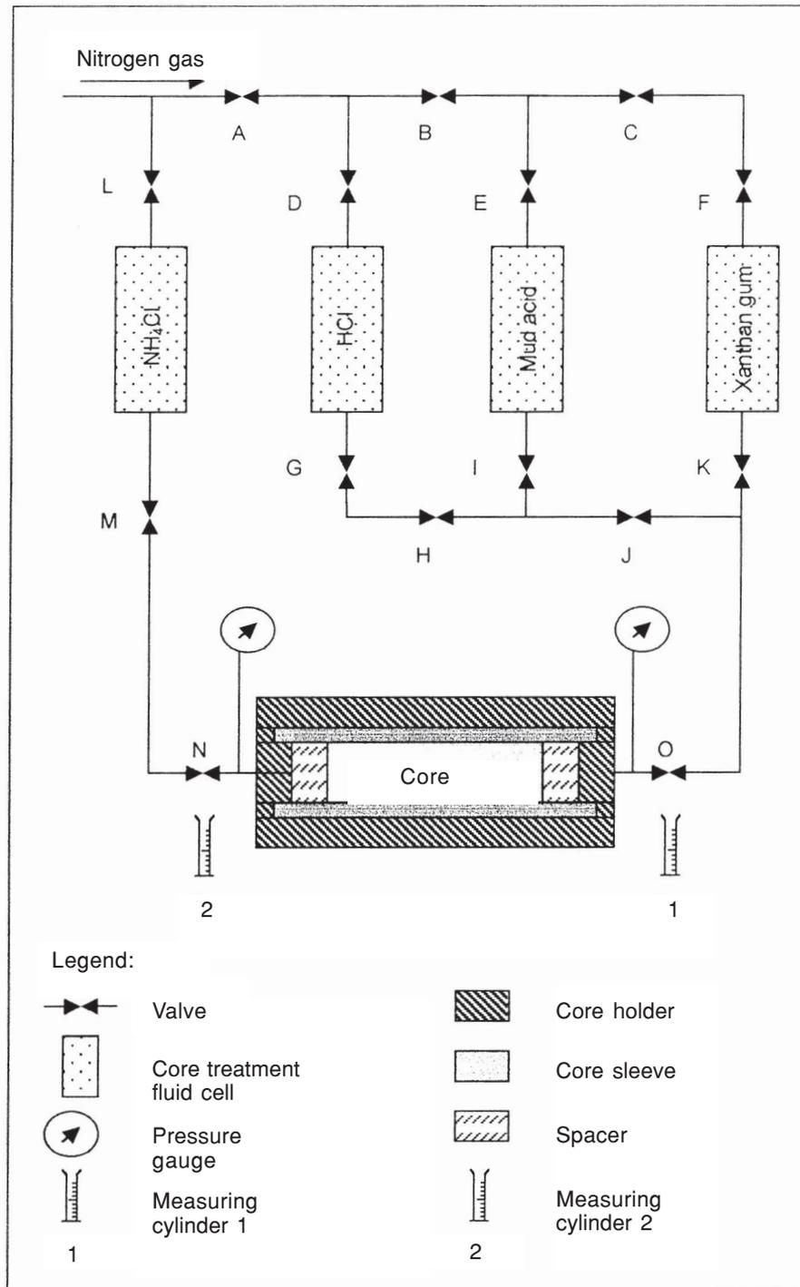
**Figure 2** Schematic diagram of the acidizing system
