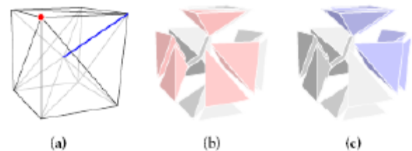
Figure 2 (b) depicts red tetrahedra that share the same red node in (a); (c) shows the tetrahedra in blue incident on the blue spring - edge in (a) [2]
