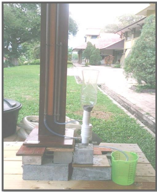
Figure 2 Prototype of falling head test for geotextile drainage capacity
