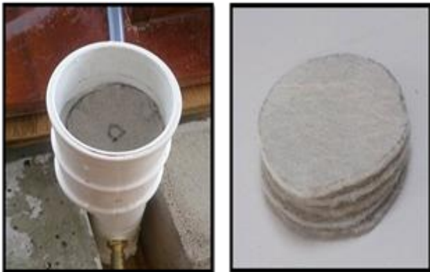
Figure 2 Prototype of falling head test for geotextile drainage capacity
