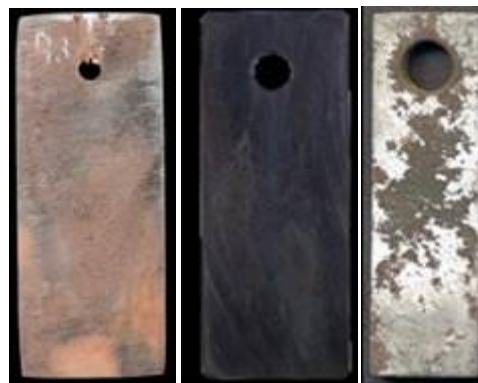
Figure 2 Carbon steel after 6 months exposure in artificial fluids; Left: MB, 150 °C; Center: SBY, 175 °C; Right: NGB, 150 °C
