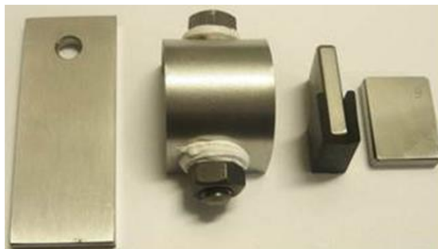
Figure 1 Specimen Design for Exposure, SCC, Crevice Corrosion and Electrochemical Tests
