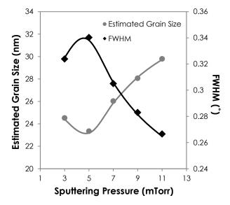
**Figure 3** The variation of full width at half maximum (FWHM) and estimated grain size of ZnO (002) diffraction peak at different sputtering pressure
