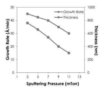
**Figure 1** Dependence of growth rate and thickness of ZnO thin films on the sputtering pressure deposited on plastic substrates and the growth time is 25 minute
