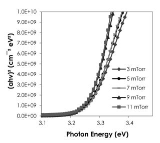
**Figure 5** Plot of graph  $(ahv)^2$  versus photon energy for ZnO films deposited on plastic substrate at different sputtering pressure
