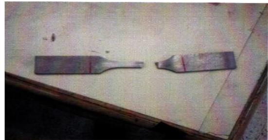
**Figure 6** Condition of specimen after failure in region of 34-48 mm, 75% UTS
