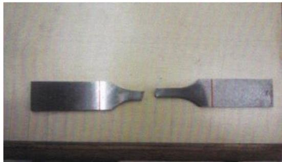
**Figure 7** Condition of specimen after failure in region of 10-12 mm, 80% UTS
