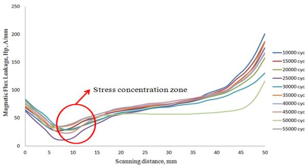
**Figure 4** Graph of magnetic flux leakage signals with scanning interval distances in 80% UTS
