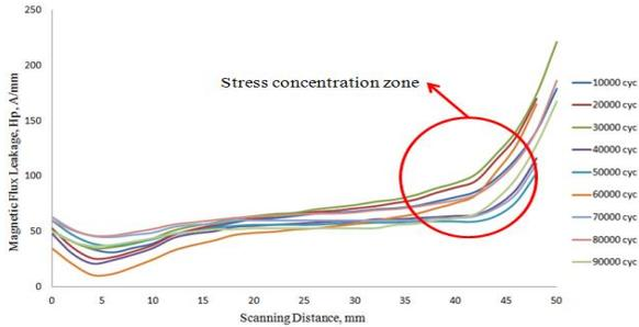
**Figure 3** Graph of magnetic flux leakage signals with scanning interval distances in 75% UTS
