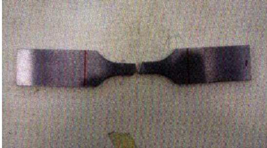
**Figure 8** Condition of specimen after failure in region of 34-42 mm, 85% UTS
