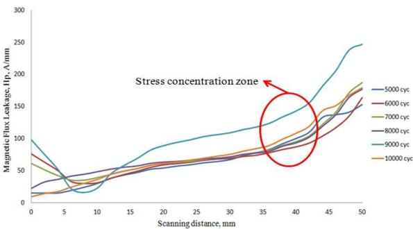
**Figure 5** Graph of magnetic flux leakage signals with scanning interval distances in 85% UTS
