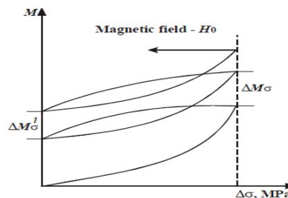
**Figure 1** Schematic diagram of magnetic memory effect (A. Dubov, 2006)
