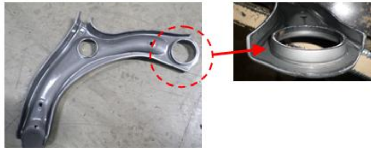
Figure 1 Hole burring of inner burring process at lower arm part
