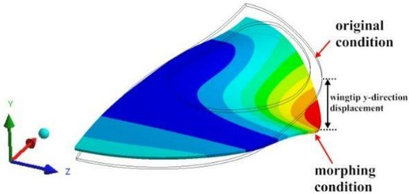
Figure 1 TM wing deformation result.
