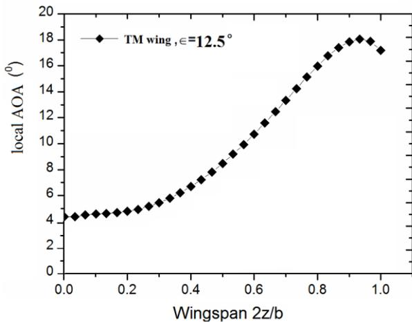
Figure 4 Local AOA (°) vs. wingspan (2z/b) graph.
