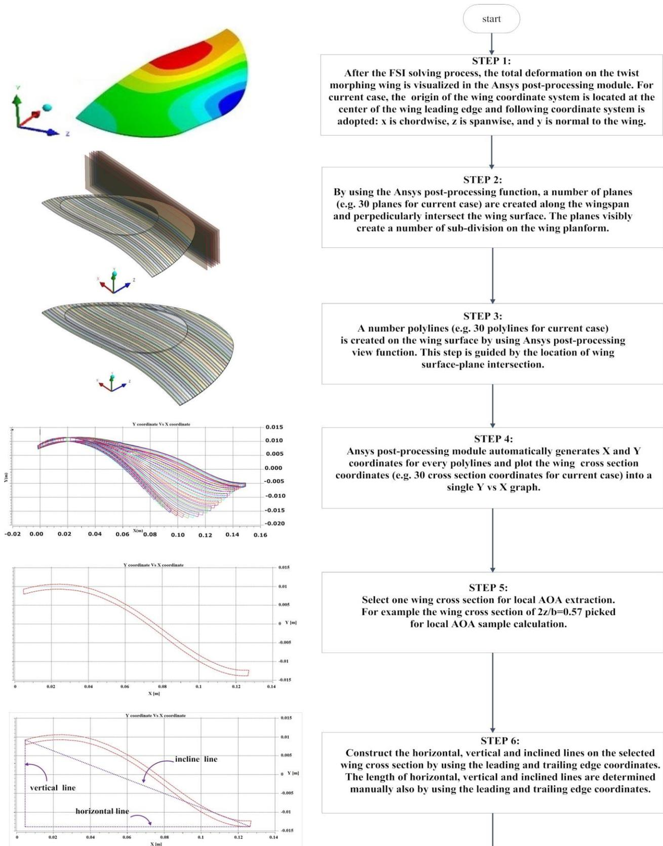
**Figure 2** The summary of local AOA extraction method for twist morphing MAV wing.
