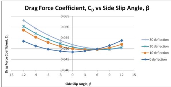
Figure 6 Drag force coefficient ( $C_D$ ) against side slip angle ( $\beta$ )
