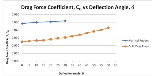
Figure 7 Drag force coefficient ( $C_D$ ) against deflection angle ( $\delta$ ) at  $\beta = 0^\circ$
