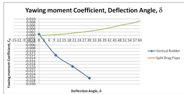
Figure 9 Yawing moment coefficient ( $C_N$ ) against deflection angle ( $\delta$ ) at  $\beta = 0^\circ$
