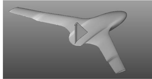
Figure 2 BWB-UAV Baseline-II with a central vertical rudder without canard
