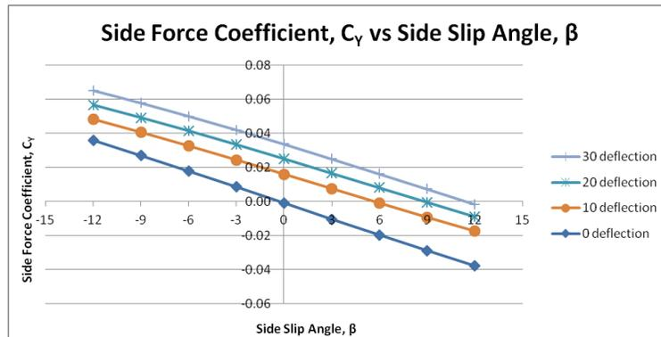
Figure 5 Side force coefficient ( $C_Y$ ) against side slip angle ( $\beta$ )
