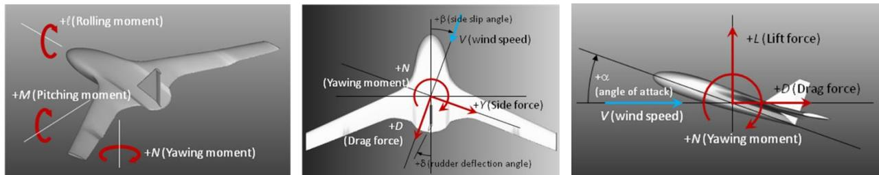
Figure 3 Sign convention for aerodynamic forces and moments
