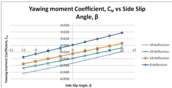
Figure 8 Yawing moment coefficient ( $C_N$ ) against side slip angle ( $\beta$ )
