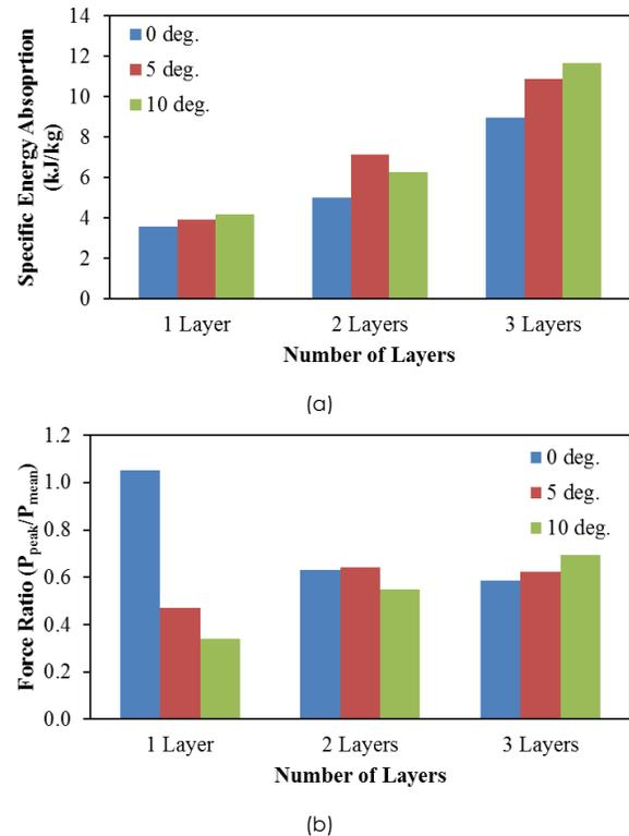
Figure 8 Effect of number of layers on the (a) specific energy absorptions and (b) force ratios
