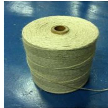
Figure 1 A bundle of an as-received kenaf yarn fibre
