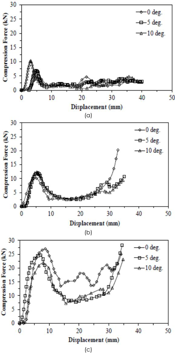
Figure 5 Crushing responses of kenaf fibre reinforced composites, (a) 1 layer, (b) 2 layers and (c) 3 layers
