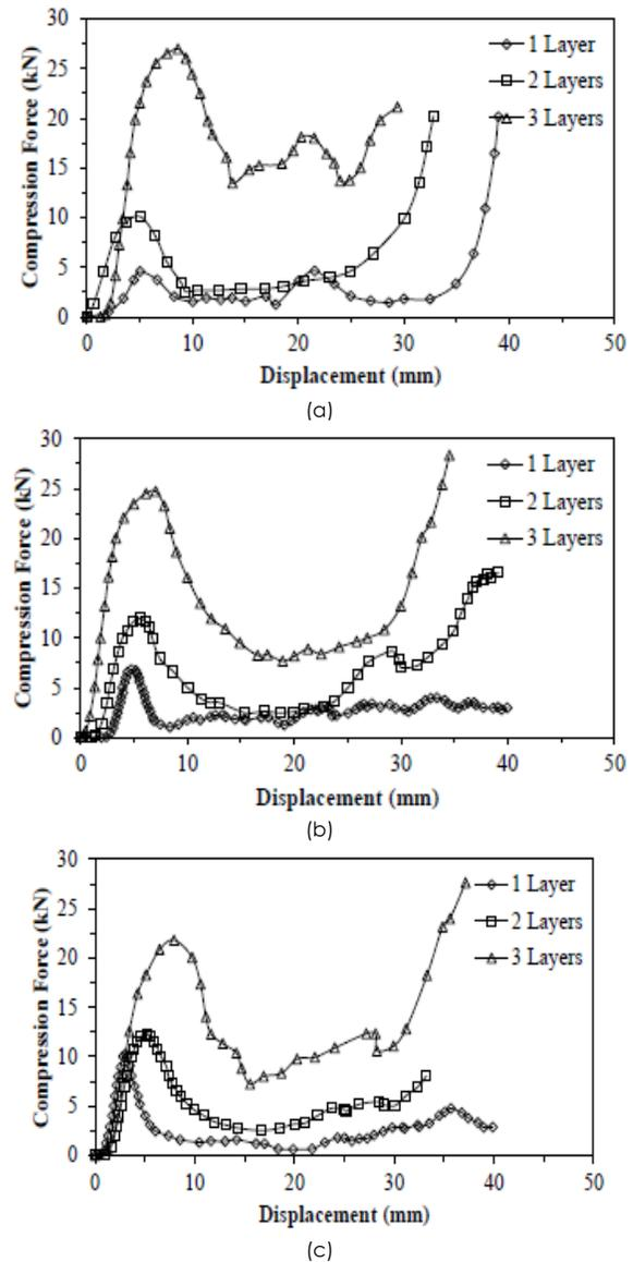
Figure 6 Crushing responses of kenaf fibre reinforced composites, (a) 0°, (b) 5° and (c) 10°
