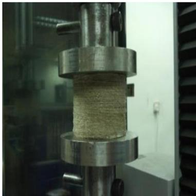
**Figure 4** Composite is laterally positioned before quasi-static compression loading
