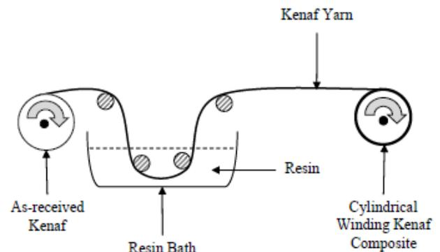
Figure 2 Schematic diagram of the winding process of the kenaf yarn fibre
