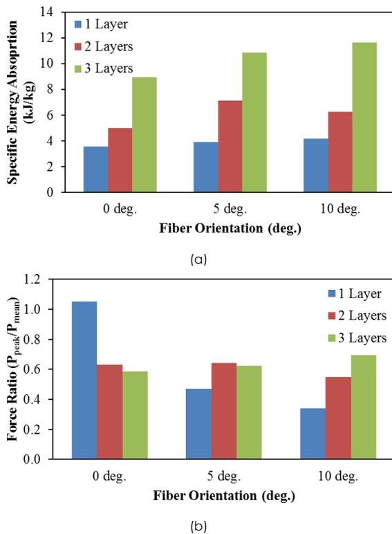
Figure 7 Effect of fiber orientations on the (a) specific energy absorptions and (b) force ratios
