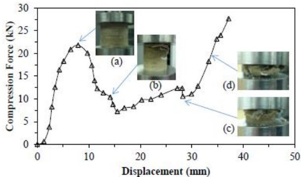
Figure 9 Failure mechanisms at different crushing levels
