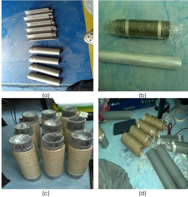
**Figure 3** (a) Plastic mould, (b) Mould assembly, (c) Kenaf yarn wrapped around the mould and (d) Final composite tubes
