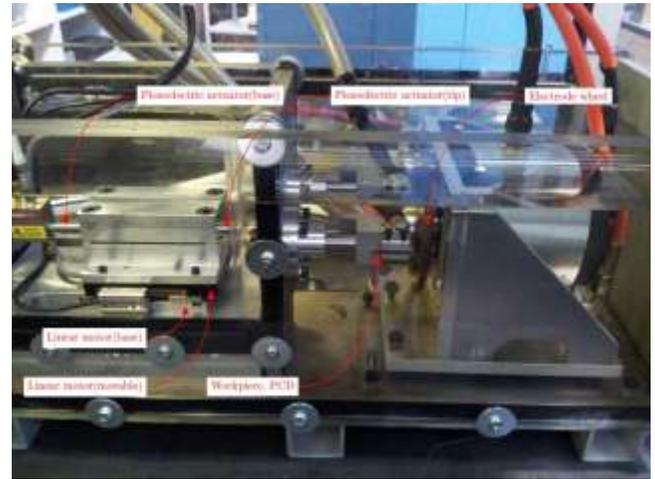
Figure 2 Electrical discharge grinding with dual stage actuators
