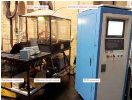
Figure 4 Sub-systems of the electrical discharge grinding
