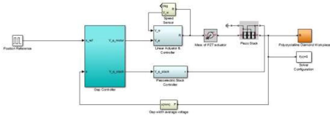
Figure 6 Simulink block diagram for the dual stage actuators
