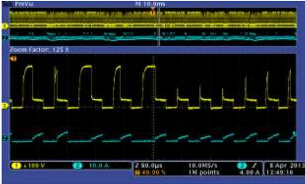
Figure 1 Pulse pattern of electrical discharge grinding
