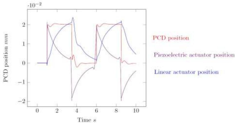
Table 7 Simulated PCD workpiece position response with dual stage actuators
