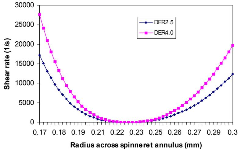
**Figure 9** Shear rate profiles in spinneret at the various dope extrusion rates for dope solution: 27% CA, 43.8% acetone and 29.2 % formamide (ratio of acetone to formamide = 1.5)
