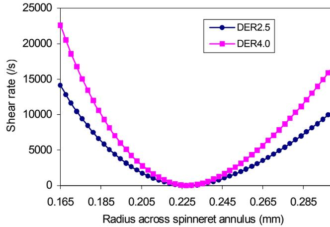
**Figure 7** Shear rate profiles in spinneret at low and high dope extrusion rates with dope solution: 25% CA, 45% acetone and 30% formamide (ratio of acetone to formamide = 1.5)
