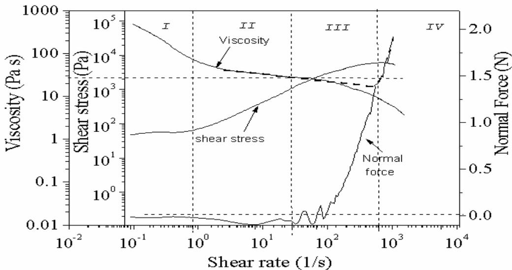
**Figure 1** Flow curve with normal force at 25°C for 25% CA, 37.5% acetone and 37.5% formamide (Ratio of acetone to formamide = 1)
