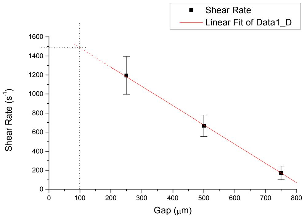
**Figure 5** Shear rate versus gap size at sample boundary (optical shear cell data)
