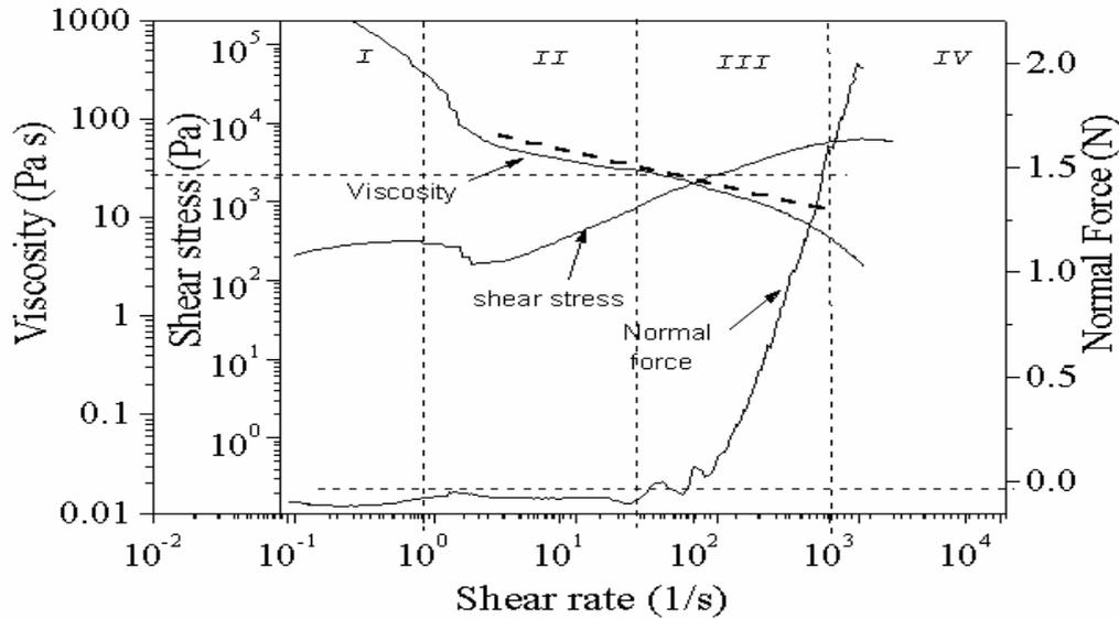
**Figure 4** Flow curve with normal force at 25°C for 27%CA, 43.8% acetone and 29.2% formamide (Ratio of acetone to formamide = 1.5)
