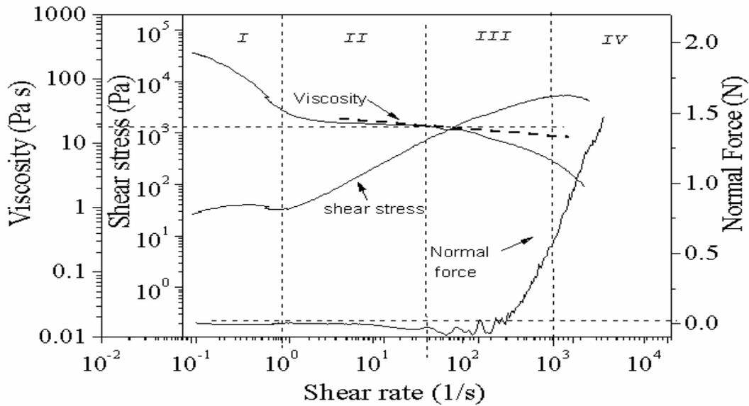
**Figure 2** Flow curve with normal force at 25°C for 25%CA, 45% acetone and 30% formamide (Ratio of acetone to formamide = 1.5)
