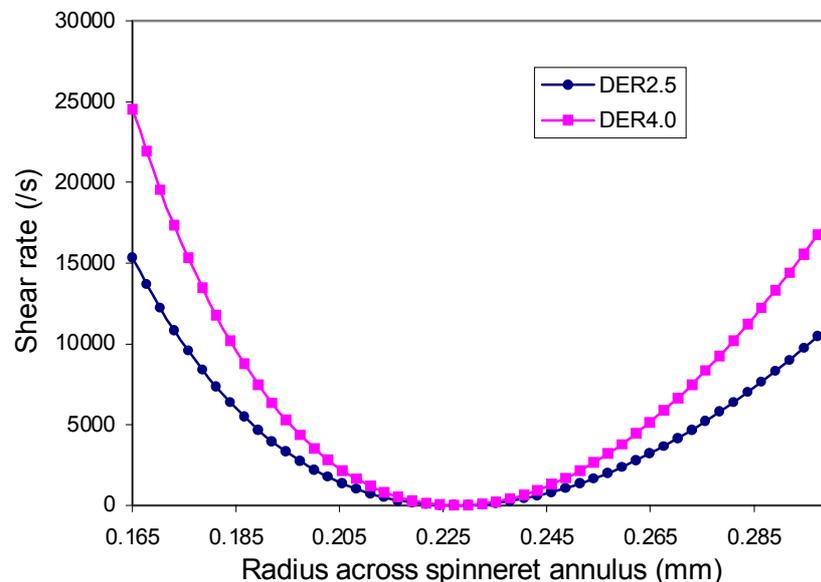
**Figure 6** Shear rate profiles in spinneret at low and high dope extrusion rates with dope solution: 25% CA, 37.5% acetone and 37.5% formamide (ratio of acetone to formamide = 1.0)
