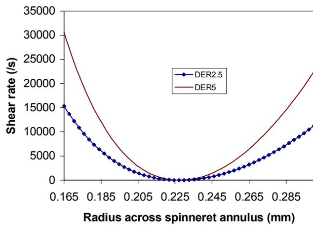
**Figure 8** Shear rate profiles in spinneret at the various dope extrusion rates for dope solution: 27% CA, 36.5% acetone and 36.5% formamide (ratio of acetone to formamide = 1.0)
