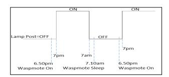
Figure 1 Timeline for sensor node operation
