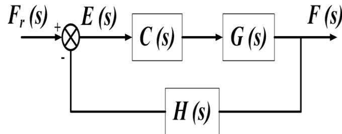
Figure 4 Closed-loop control system for path force control in FSW
