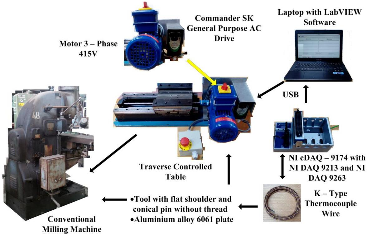
**Figure 2** System integration of a FSW machine with a traverse controlled table
