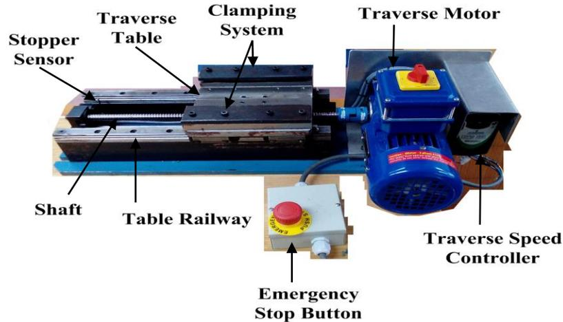
Figure 3 Traversal controlled table configuration
