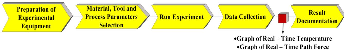
Figure 1 Experiment flowchart for temperature and path force analysis in FSW
