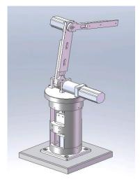
Figure 1 The configuration of the variable link length 3 DOF revolute articulated Manipulator
