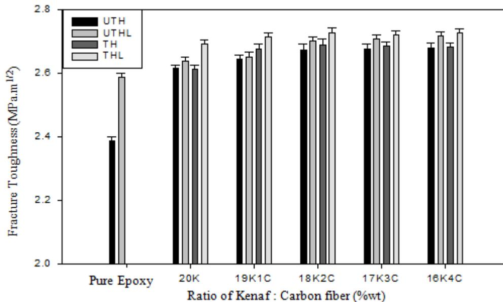
Figure 3 Fracture toughness of epoxy reinforced hybrid kenaf/carbon fiber composite
