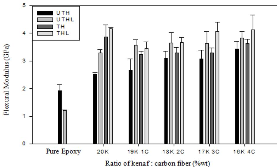
Figure 2 Flexural modulus of epoxy reinforced hybrid kenaf/carbon fiber composite
