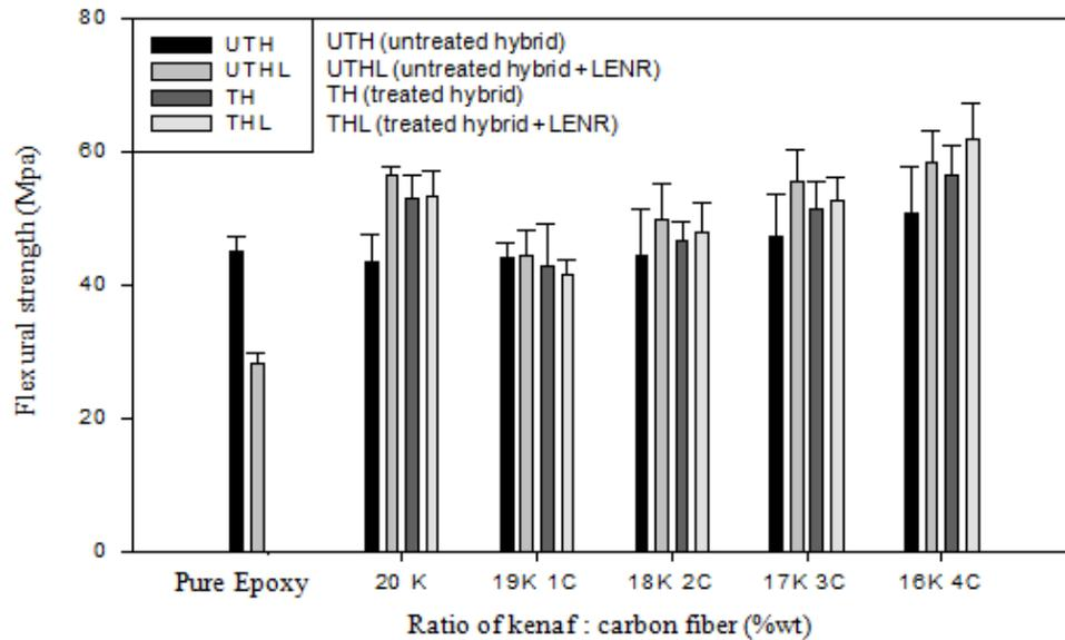
Figure 1 Flexural strength of epoxy reinforced hybrid kenaf/carbon fibre composite
