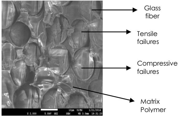
**Figure 3** FESEM microstructure showing crack propagation of nanommodified GFRP composites observed under 2000x magnification.
