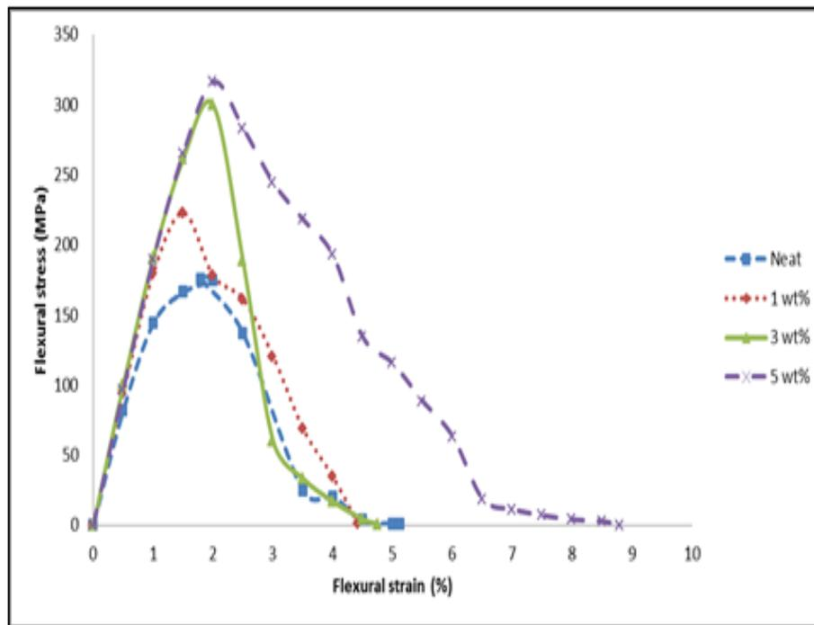
**Figure 1** Typical flexural stress-strain curves of nanomodified (GFRP) composites system
