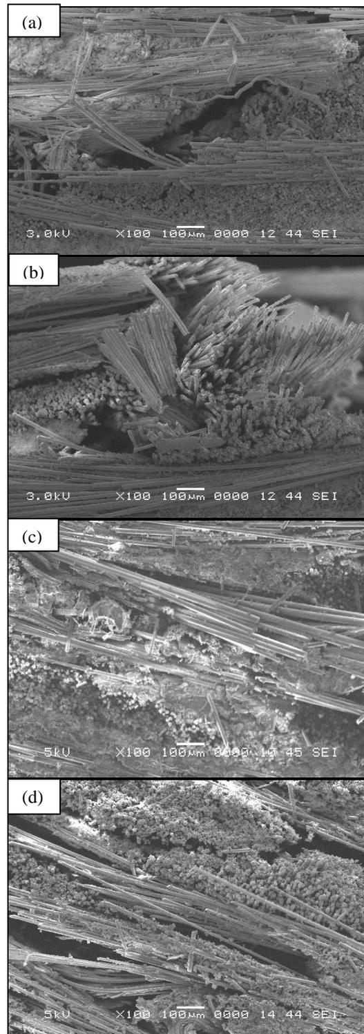
**Figure 2** FESEM examination on fracture surface of GFRP (a) neat system; (b) 1 wt% nanoclay; (c) 3 wt% nanoclay; (d) 5 wt% nanoclay
