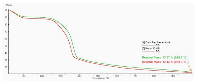
Figure 1 TGA analysis of Kapur and Dark Red Meranti samples
