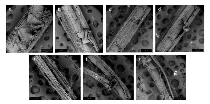
Figure 2 Morphology of single mengkuang fiber before and after each extraction process: (a) 0% Treatment (b) 2% NaOH at 60 min (c) 2% NaOH at 120 min (d) 6% NaOH at 60 min (e) 6% NaOH at 120 min (f) 10% NaOH at 60 min (g) 10% NaOH at 120 min (all magnification at 50x)
