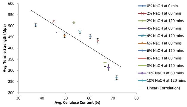
Figure 1 The relationship between cellulose content and tensile strength of continuous single fiber
