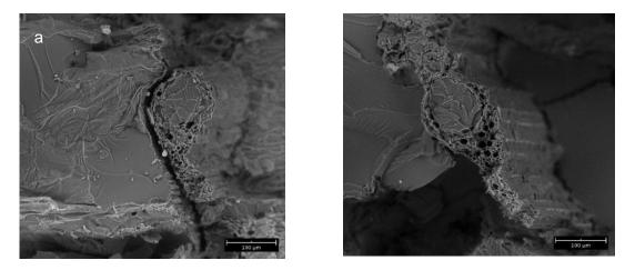
Figure 3 Morphology of the fracture surface of the continuous Mengkuang fiber composite. (Magnification of 500x)
