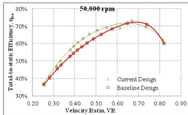
Figure 8 Comparison of VR between current and previous design at 100% design speed
