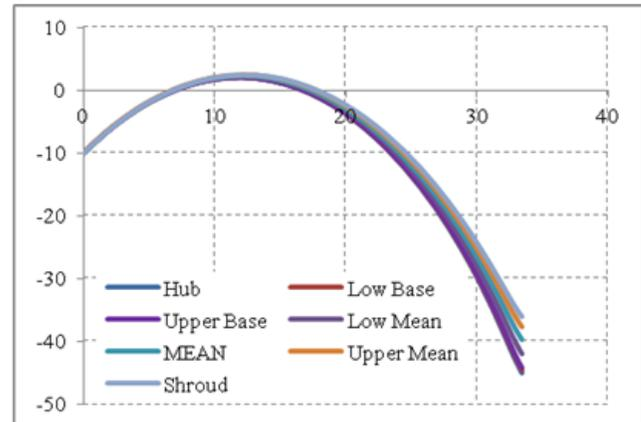
Figure 3 Camberline angle for blade profile
