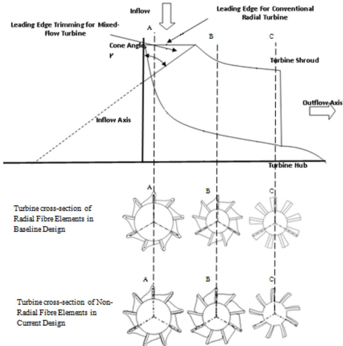
Figure 1(a) Schematic diagram of the fibre elements utilized in the Baseline Design and Current Design [3]
