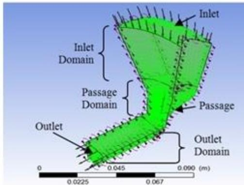
Figure 4 Meshing of the turbine and boundary interface
