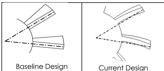
Figure 1(b) Enlarged cross-sectional view of the blades at trailing edge (C)
