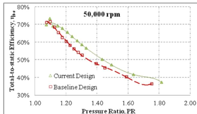
Figure 6 Comparison of  $\eta_{t-s}$  between current and previous design at 100% design speed
