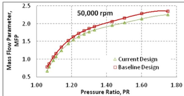
Figure 10 Comparison of MFP vs PR between current and previous design
