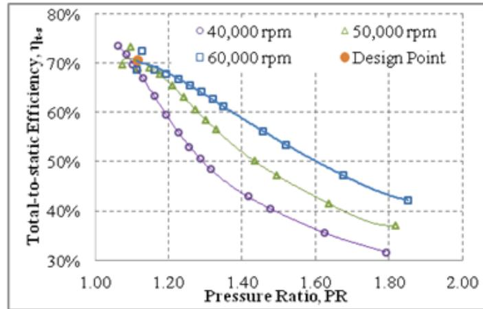
Figure 7  $\eta_{ts}$ -vs PR for current design
