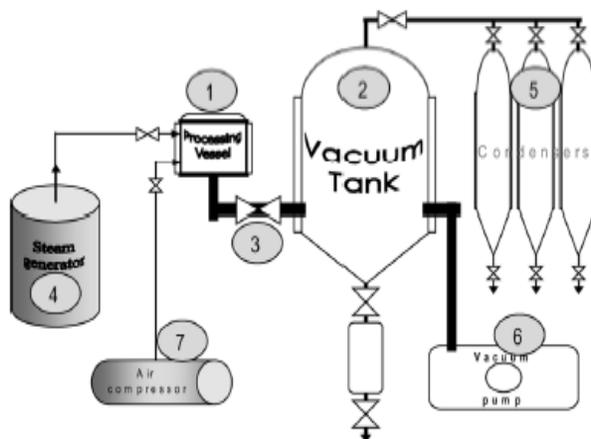
**Figure 1** Schematic presentation of DIC machine: 1. Processing chamber; 2. vacuum tank; 3. controlled instant pressure drop valve; 4. Steam generator; 5. condensers; 6. vacuum pump; 7. air compressor
