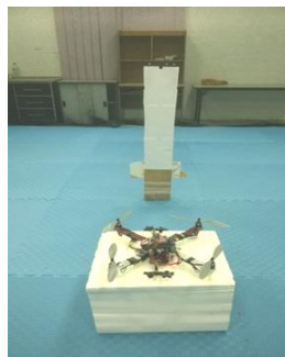
Figure 4 Experimental setup for evaluation of sensor performance
