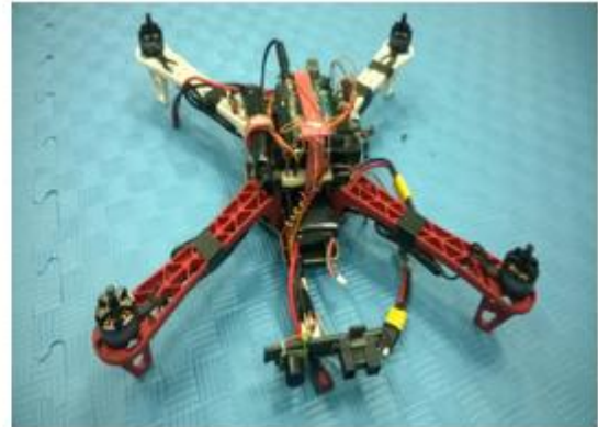
Figure 3 Quadrotor platform with on-board sensors and microcontroller board
