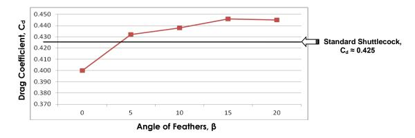
Figure 4 Drag coefficient,  $C_d$ ; versus angle of feathers,  $\beta$
