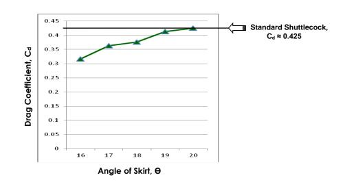
Figure 2 Drag coefficient, Cd versus angle of skirt, O
