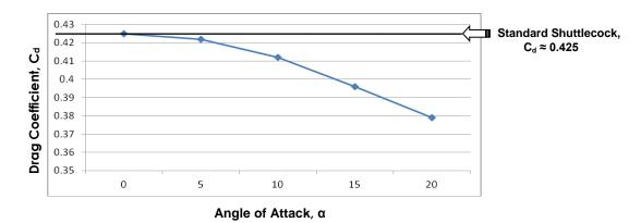
Figure 3 Drag coefficient,  $C_d$ ; versus angle of attack,  $\alpha$
