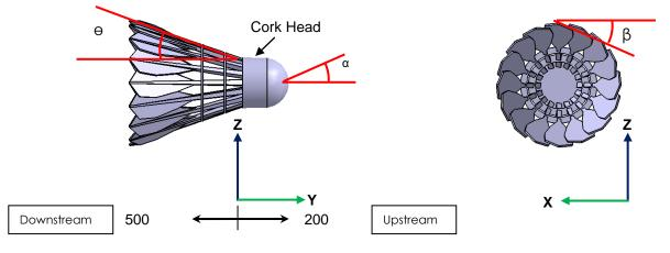
Figure 1 Angle of attack,  $\alpha$ ; angle of skirt,  $\Theta$ ; and angle of feather,  $\beta$ ; of a standard shuttlecock
