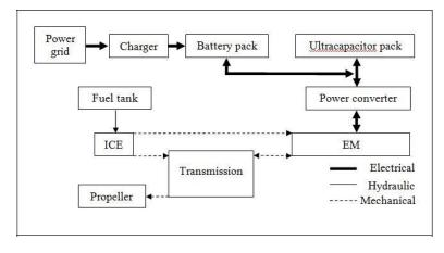
Figure 1 Schematic illustration of series-parallel PHERB powertrain
