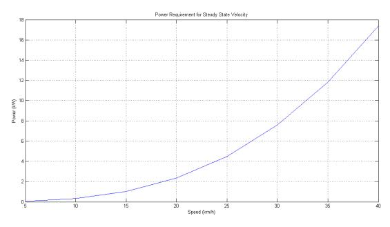
Figure 2 Boat power requirements for steady state velocity
