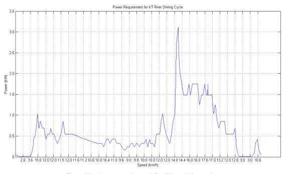
Figure 4 Boat power requirements for KT river driving cycle
