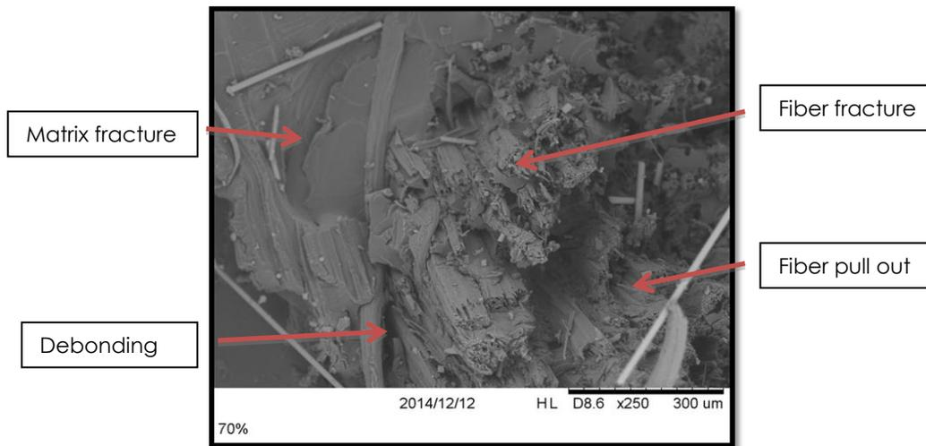
Figure 4 SEM microstructure of fatigue specimen
