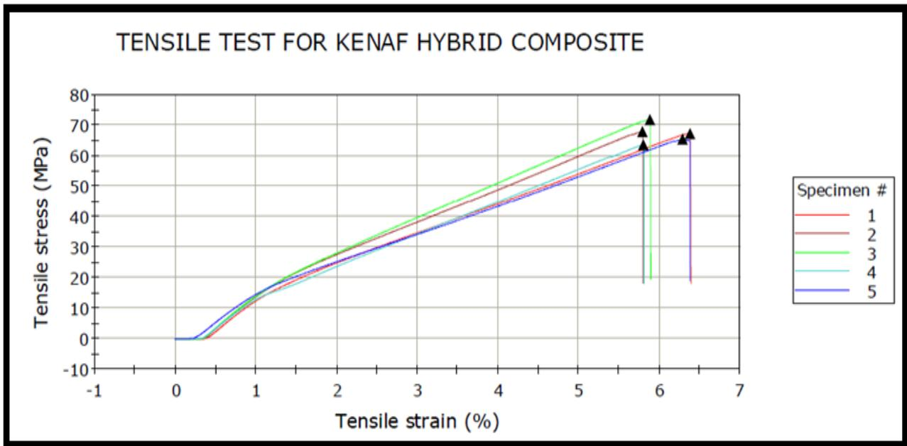
Figure 3 Graph of Tensile Stress (MPa) against Tensile Strain (%)
