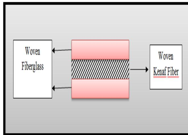
Figure 1 Arrangement of woven kenaf fiberglass hybrid composite
