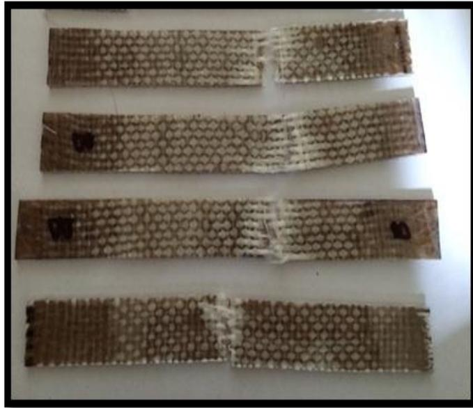
Figure 2 Specimens after tensile test
