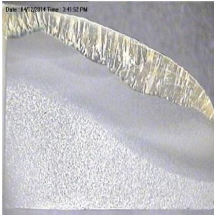
**Figure 3 (a)** Macrostructure of RE115 Rail Welded with Magna 488-Rail
