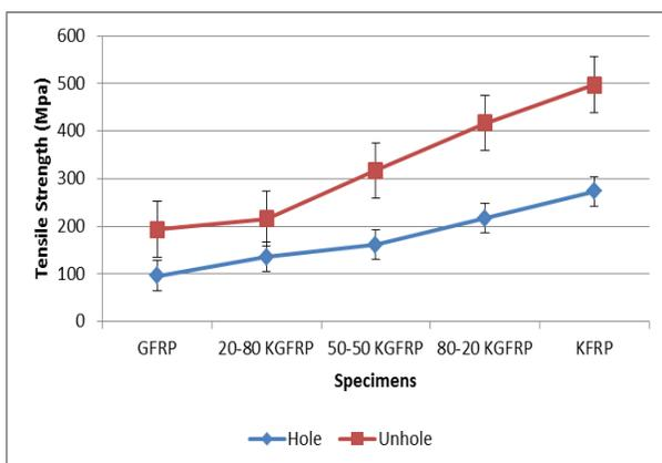
**Figure 1** Effect of hybridization Kevlar fiber to glass fiber on tensile strength
