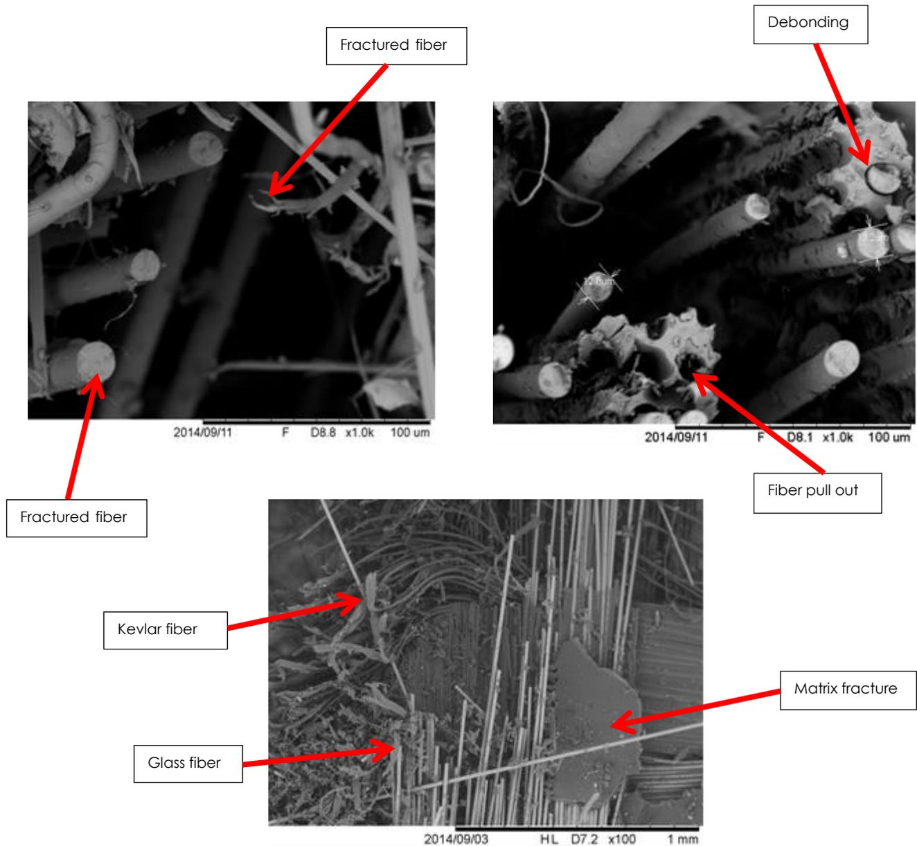
Figure 3 Microscopic observation of fractured surface of Kevlar/glass fiber hybrid composite laminates
