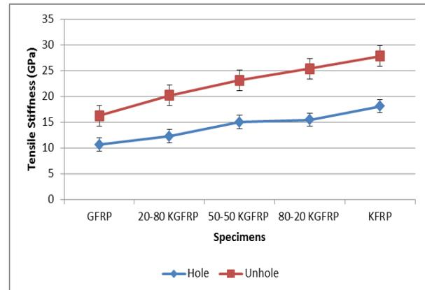
**Figure 2** Effect of hybridization Kevlar fiber to glass fiber on tensile stiffness
