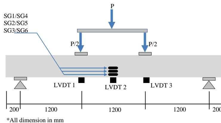
Figure 2 Experiment setup
