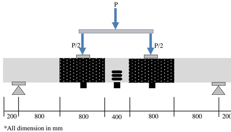
Figure 3 Application of CFRP on BRTB-R
