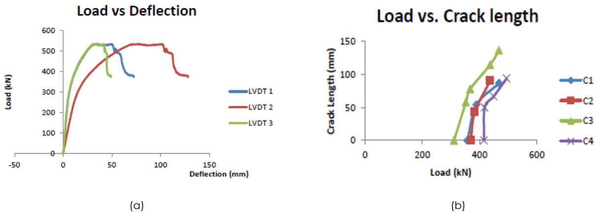
Figure 4 (a) Load-deflection curves of PRTB-C (b) Load-crack length curves of PRTB-C
