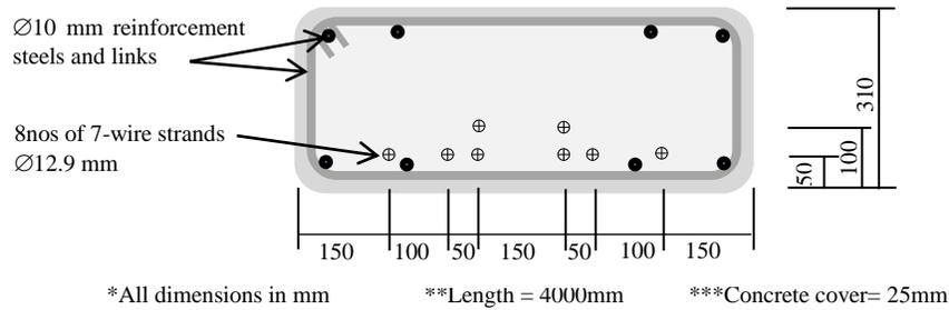
Figure 1 Tendons arrangement in PRTB-C and PRTB-R
