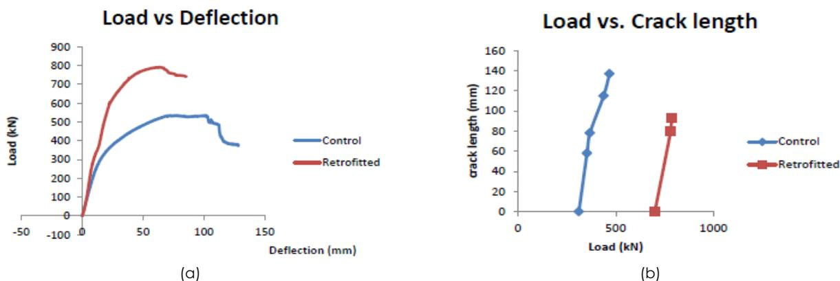
**Figure 6** (a) Comparison of Load-Deflection curve of PRTB-C and PRTB-R (b) Comparison of significant crack length of PRTB-C and PRTB-R
