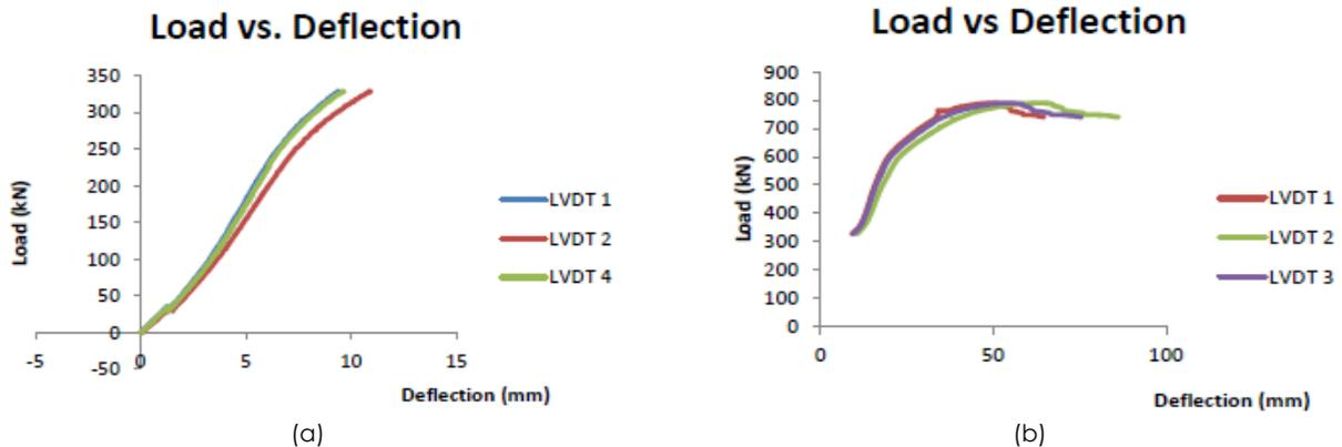
Figure 5 (a) Load-deflection of PRTB-R before retrofit (b) Load-deflection of PRTB-R before retrofit
