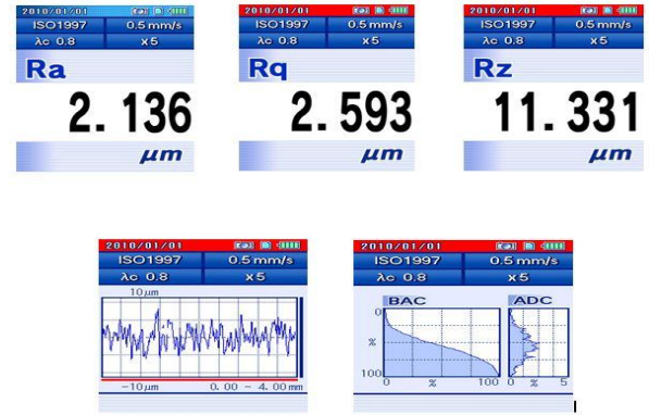
Figure 4 Surface roughness data at 1.0 mm depth of cut for different ultrasound frequencies
