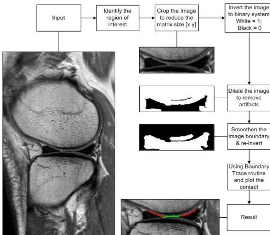
**Figure 2** A MATLAB's script process flow; red pixels represent as contact length between femoral cartilage and meniscus, while green pixels are the contact length between femoral and tibial cartilages
