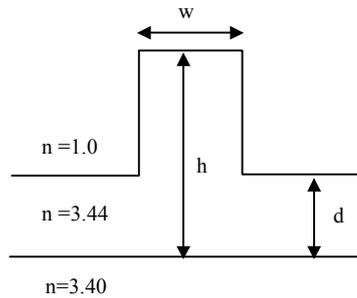
**Figure 7** Schematic diagram of the GaAs waveguide structure operating at 1.15  $\mu\text{m}$
