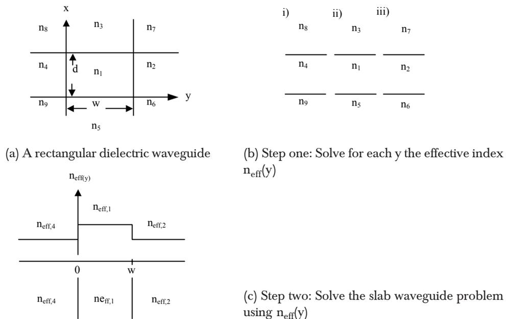
**Figure 4** (a) A rectangular dielectric waveguide to be solved using the effective index method. (b) Solve the slab waveguide problem for each  $y$  and obtain effective index profile  $n_{\text{eff}}(y)$ . (c) Solve the slab waveguide problem with the effective index problem  $n_{\text{eff}}(y)$
