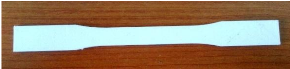
Figure 1 Printed tensile specimen fabricated via desktop 3D printer
