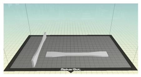
Figure 1 Orientation of specimens visualized in Makerware
