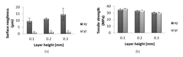
Figure 2 Effect of layer height and printing orientation on (a) surface roughness, (b) tensile strength.
