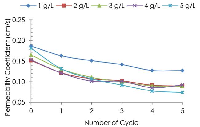
**Figure 9** Relationship between permeability and number of cycles of clogging materials from highway
