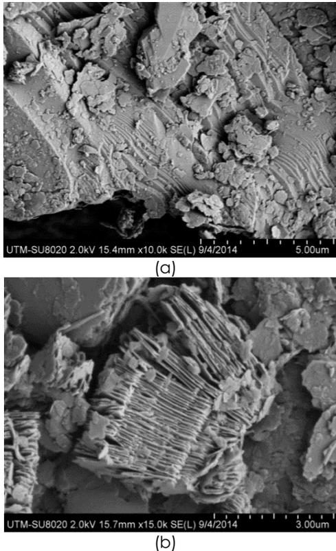
**Figure 3** Surface texture for clogging materials at magnification of 5µm and 3 µm for (a) highway and (b) residential
