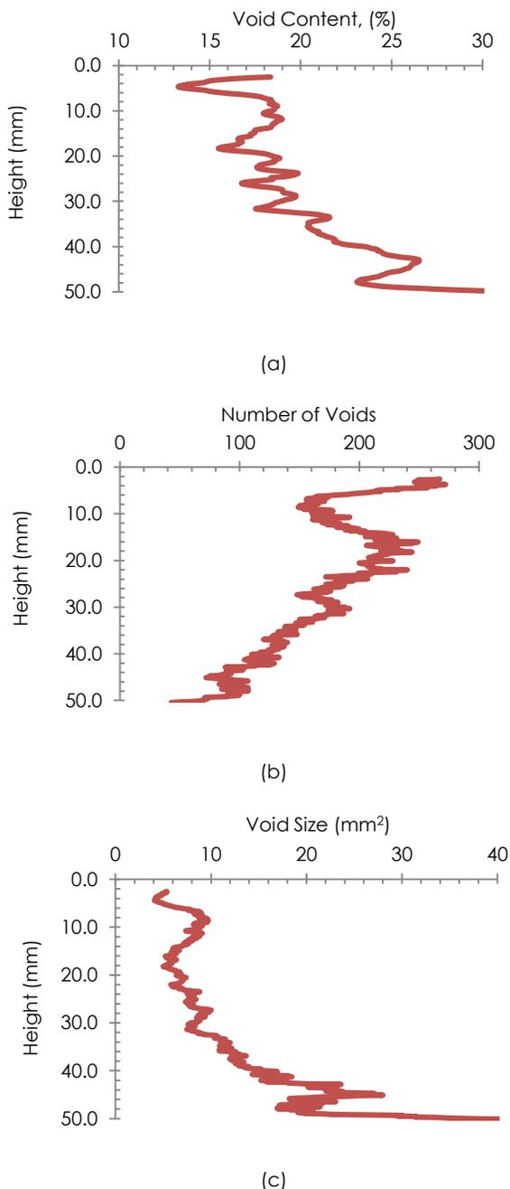
**Figure 8** Air Voids Distribution For Porous Asphalt Mixtures (a) Voids content; (b) Voids Number; (c) Voids Size
