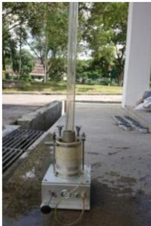
**Figure 6** Falling-head permeameter
