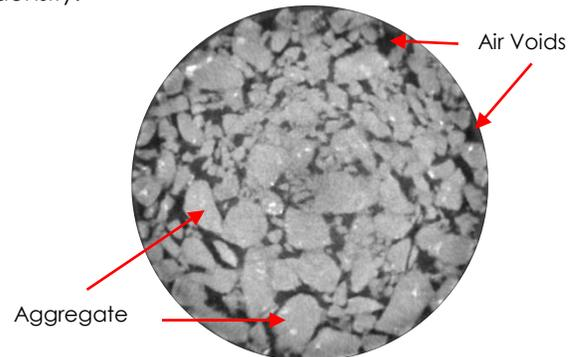
**Figure 7** Two dimensional (2D) image of X-ray CT image for porous asphalt mixture
