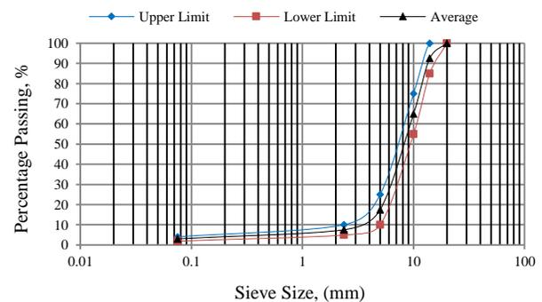
**Figure 1** Malaysian gradation limits for porous asphalt mixtures, Grading
