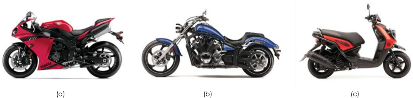
Figure 6 (a) a Class 2 Type A cockpit design motorcycle, the motorcycle featured is the 2012 Yamaha YZF R1 with, (b) a Class 2 Type B cockpit design motorcycle, the motorcycle featured is the 2014 Yamaha Stryker, and (c) a Class 1 cockpit design motorcycle, the motorcycle featured is the 2012 Yamaha Zuma 125 [4]
