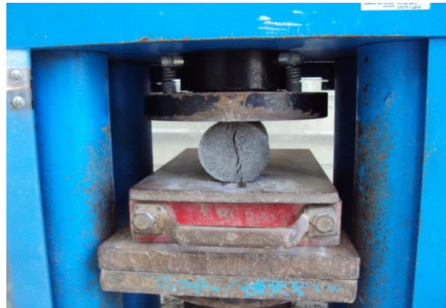
Figure 11 Tensile strength samples
