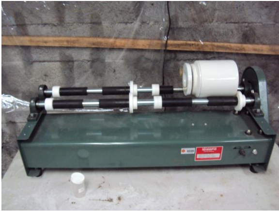
Figure 1 Grinding machine (Simpo's PTA-01)
