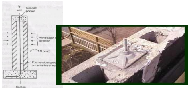
a) Post-tensioned masonry diaphragm walls
