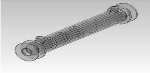
Figure 6 Developed design: 5 baffle arrangement
