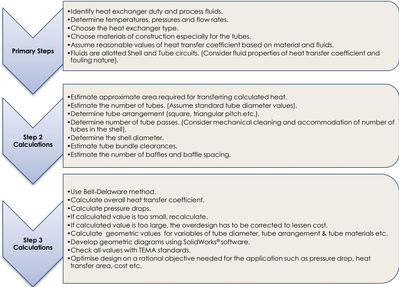
Figure 2 Methodology steps for heat exchanger designs
