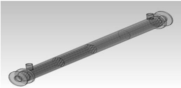
Figure 5 Developed design: 3 baffle arrangement
