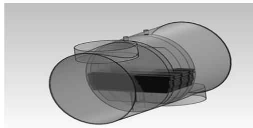
Figure 4 Optimised heat exchanger for shipboard use (part tube stack shown)
