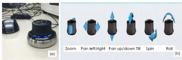
Figure 2 (a) Mouse and SpaceNavigator, (b) Six kinds of operations of SpaceNavigator.
