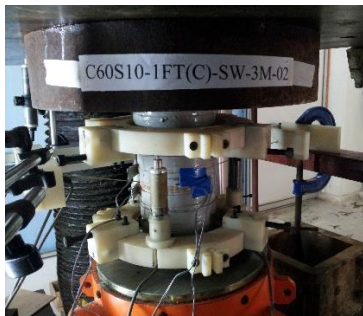
Figure 3 Diagram for strain measuring equipment and the loading device (TINIUS OLSEN Super "L" Universal Testing Machine)
