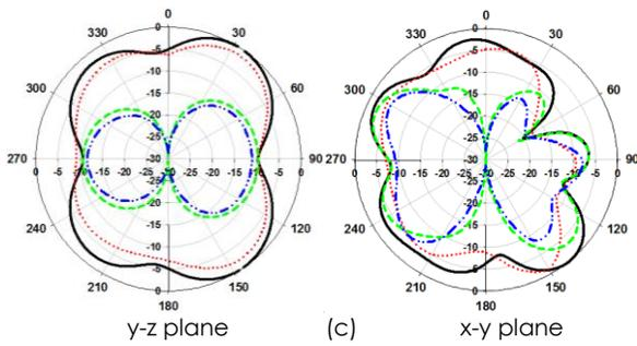
Figure 7 Simulated and measured radiation patterns of port 2 (a) ON-ON (b) OFF-ON (c) ON-OFF states.
