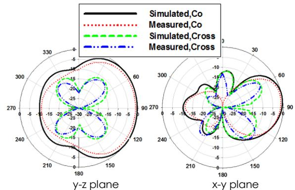
**Figure 6** Simulated and measured radiation patterns of port 1
