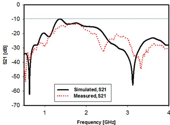
**Figure 5** Simulated and measured S21
