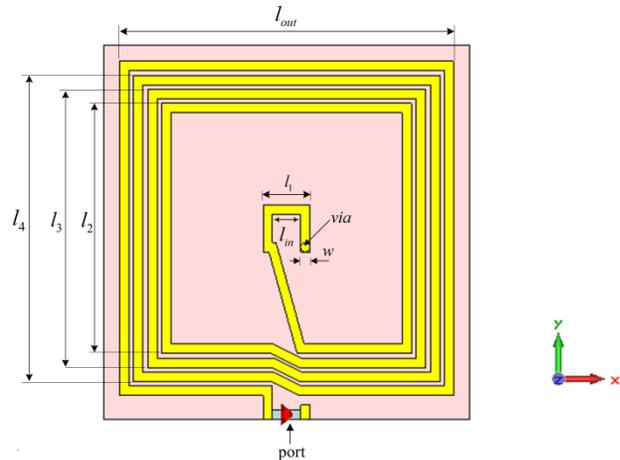
**Figure 7** Dimensions of 5-turn distributed-turns coil antenna. For the peripheral-turns design, all turns are concentrated along the coil perimeter and spaced by  $s_{min}$ . The single-turn design consists of the outermost turn only.
