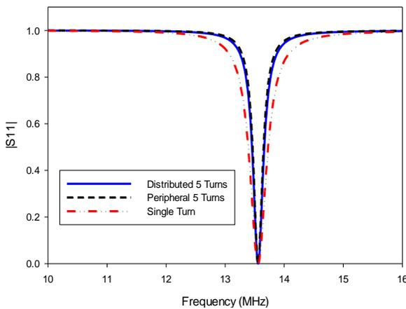
**Figure 5**  $|S_{11}|$  comparison between single-turn and 5-turn peripheral and distributed designs.
