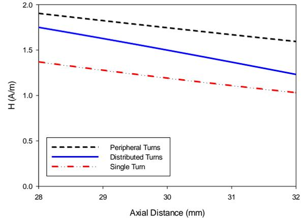
**Figure 1** Comparison of H-field magnitude for single-turn and 3-turn peripheral and distributed designs
