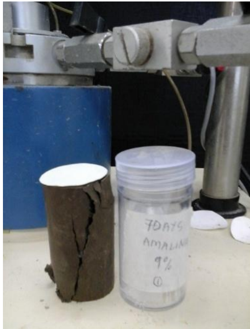
Figure 7 Specimen of UCS test
