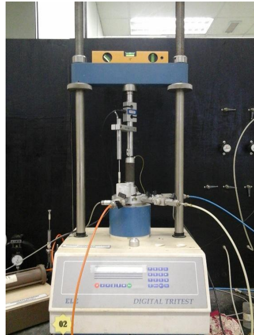
Figure 3 Unconfined Compressive Strength Test machine
