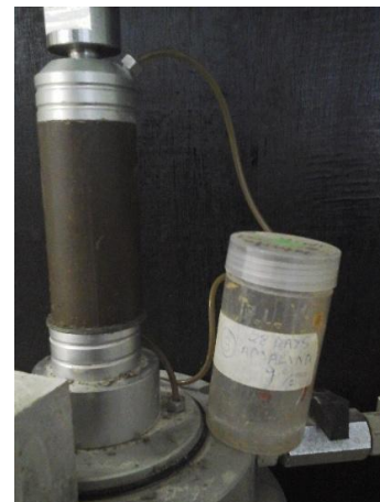
Figure 4 Clay soil specimen mixed with Biomass silica
