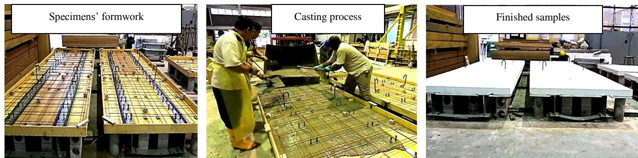
Figure 2 Full-scale test specimens preparation
