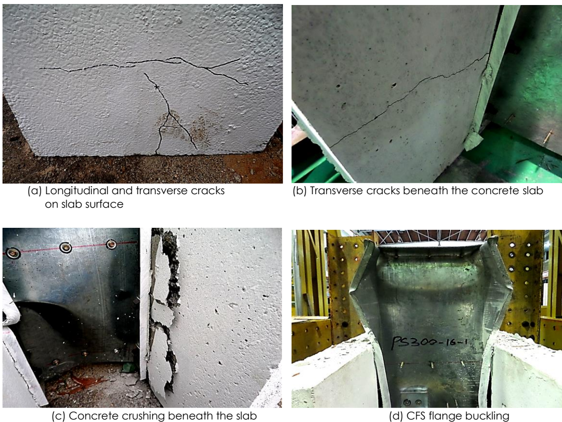
Figure 6 Failure modes of push-out test specimens
