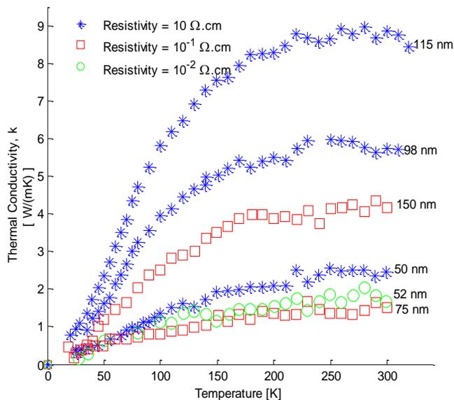
**Figure 8** Thermal conductivity versus Temperature of a SiNWs produced on different resistivity of Silicon wafer which associates with the doping concentration [30]
