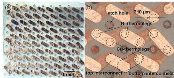
Figure 5 Microscopic image of thermoelectric device. (a) 90 Cu-Ni thermocouples fabricated on polymer. (b) Enlarge image of the thermocouples [26]. Copyright 2006, Elsevier
