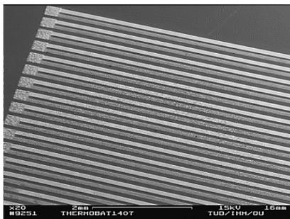
**Figure 6** A part of thermoelectric module with Sb-Bi pairs [27]. Copyright 2001, IOP Publishing
