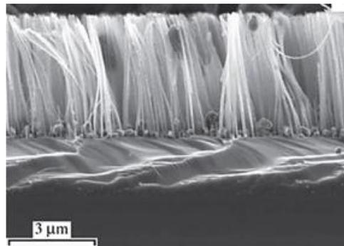
**Figure 7** SEM image of Silicon Nanowires created from metal-assisted chemical etching (MACE) process [33]. Copyright 2010, Wiley
