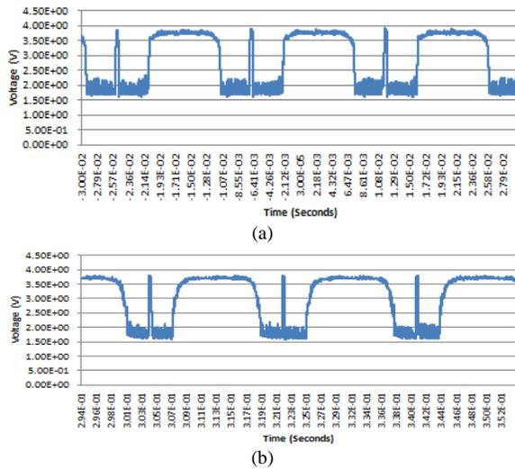
**Figure 7** CCD measurement graph for (a) 5 cent and (b) 10 cent using LED
