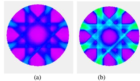
**Figure 15** Image Reconstruction for 10 cent (a) LED (b) laser diode
