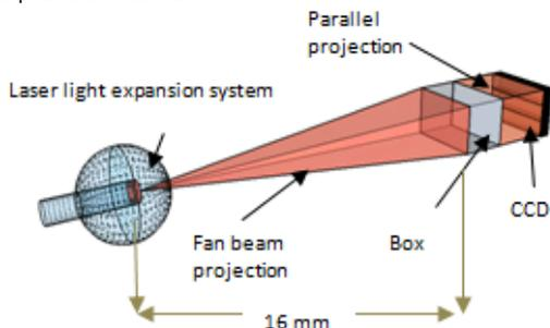
Figure 3 Mechanical design of laser beam projection
