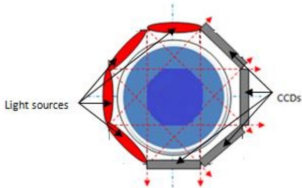
**Figure 13** Illustration of sensor orientation for image reconstruction
