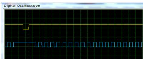
Figure 2 ROG and clock pulse generator for CCD Sony ILX551A
