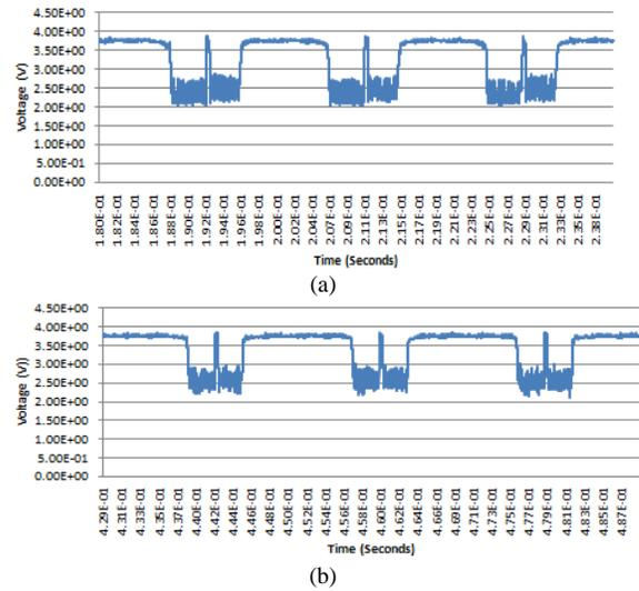
**Figure 8** CCD measurement graph for (a) 5 cent and (b) 10 cent using laser diode
