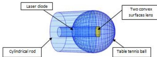
Figure 4 Laser diode light expansion system
