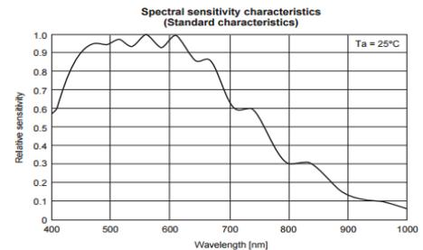
Figure 1 Spectral sensitivity graph Sony ILX551A [20]
