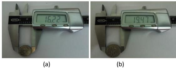
**Figure 6** Results for (a) 5 cent diameter and (b) 10 cent diameter using Vernier Caliper
