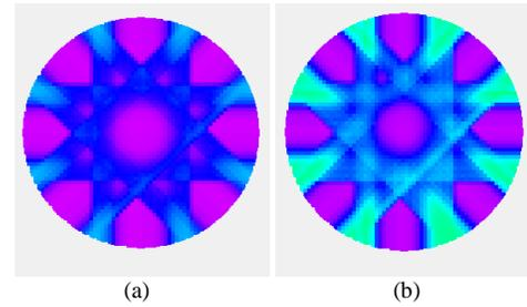
**Figure 14** Image Reconstruction for 5 cent (a) LED (b) laser diode
