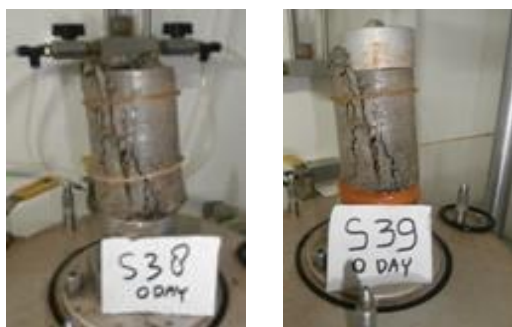
Figure 20 Joint roughness effect around failure plane on unsaturated Semarang-Bawen clay shale from triaxial test
