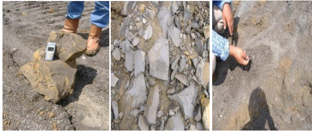
Figure 1 Changes in physical form of clay shale over time [1]
