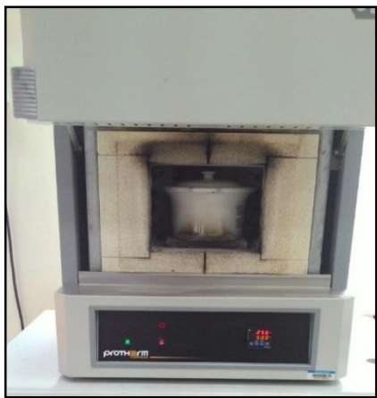
Figure 1 Sugarcane Bagasse burning process in the furnace
